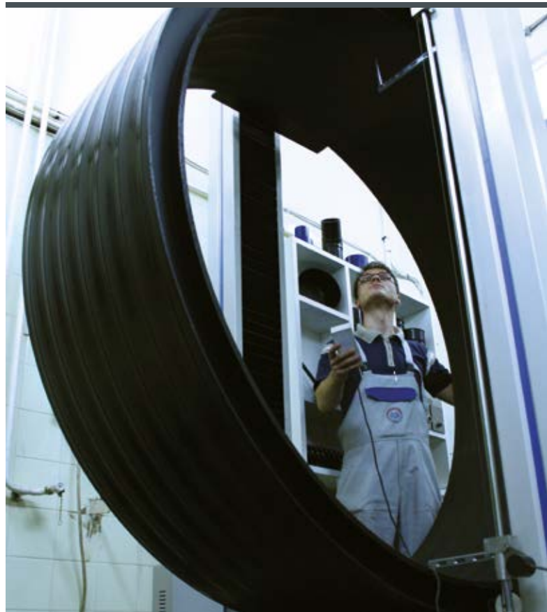
RING STIFFNESS / RING FLEXIBILITY
