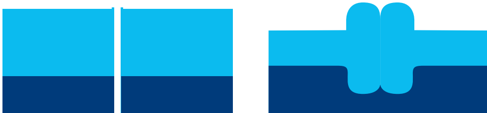
Pipe alignment and joining, beads appear under pressure
